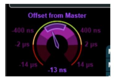
If the offset is too big or the jitter range is too big, the client cannot synchronize. You can increase the tolerance of the V\_line in "Settings" >"Switch" > "PTP" > "Timing Precision" (set to "custom" and enter a new acceptable value). Please keep in mind that this only increases the tolerance of the V\_Line; it doesn't make the PTP better. The unit may still run into trouble with other devices with a lower tolerance level.
