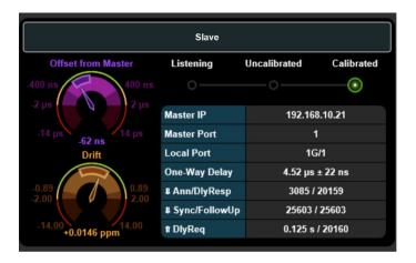
The client should be sending out messages ("Ann/DlyResp", etc. increasing). Once the client has successfully synchronized to the master's time, it will be in state "Calibrated".
