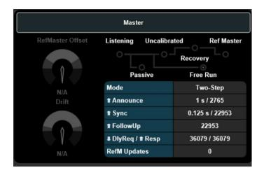
The master should send out messages ("Announce", "Sync", etc. increasing). If the master is not synchronized to an analog reference, it should be in state "Free Run", else in state "Ref Master".
