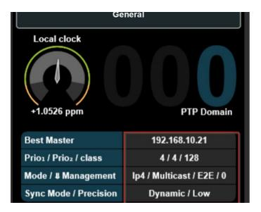
You might see the switches IP address here, if the switch runs in Boundary Clock mode. Check the client's state:
