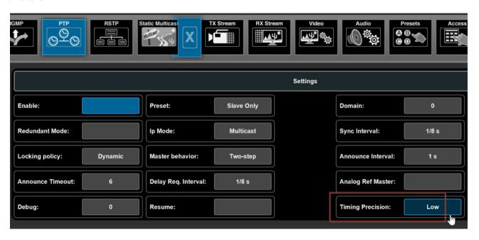
Values of  $\pm 5\mu s$  offset have been tested successfully between 2 V\_lines without impact to the video on the output. Results with other devices may vary.
